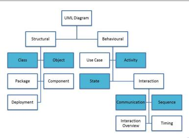
Class diagram is UML structure diagram which shows structure of the designed system at the level of classes and interfaces, shows their features, constraints and relationships - associations, generalisations, dependencies, etc.
